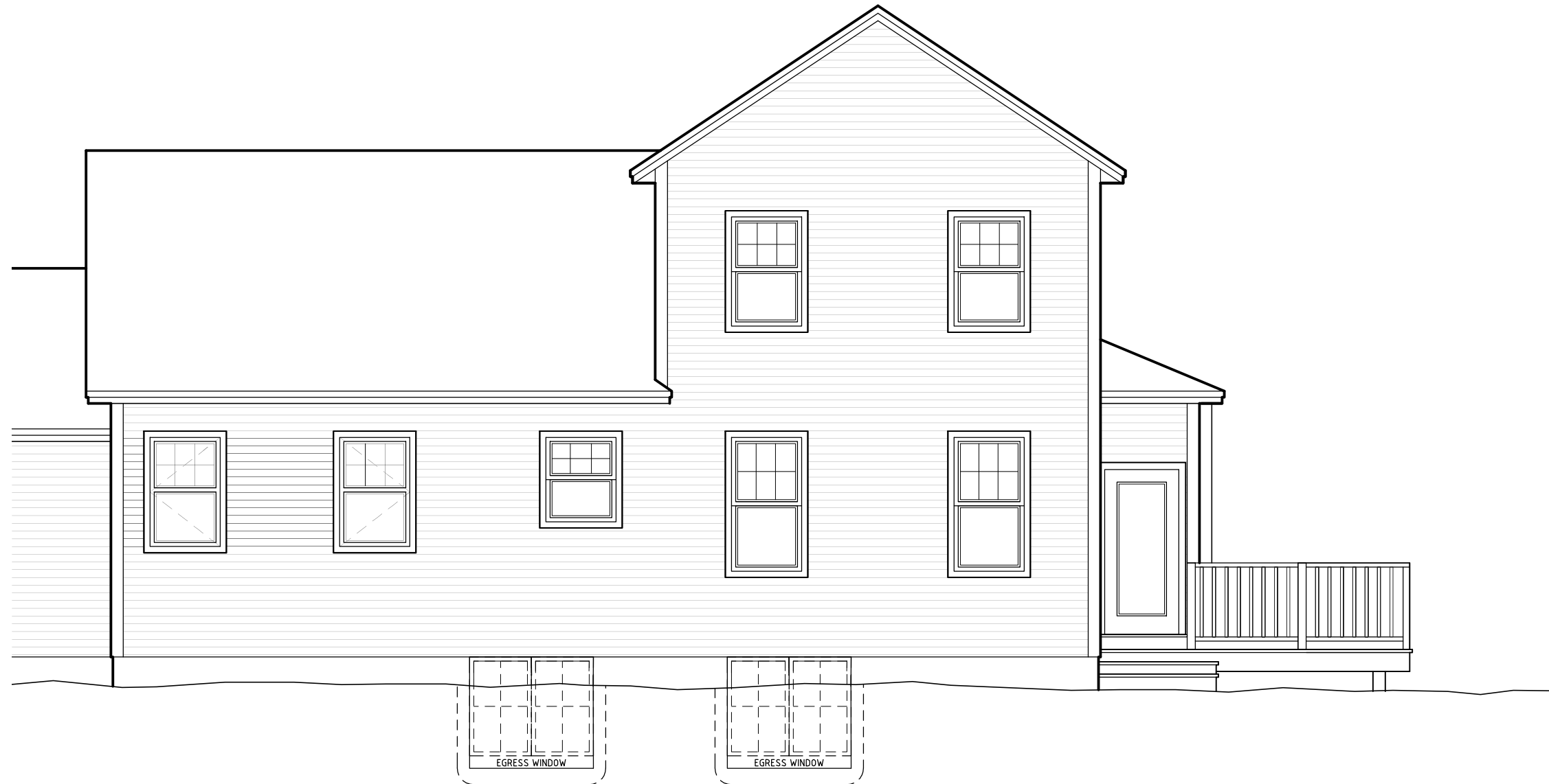
○ REAR ELEVATION SCALE: 3/16" = 1'-0"
